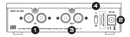
1 Connect your source to the Magni's "IN" RCA jacks with high-quality RCA cables.
